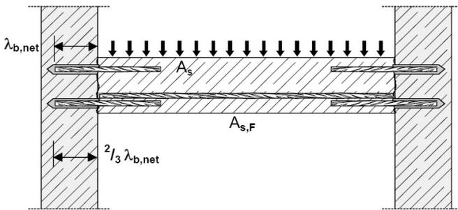
**Figure A4:** Rebar connection for components stressed primarily in compression. The rebars are stressed in compression.
