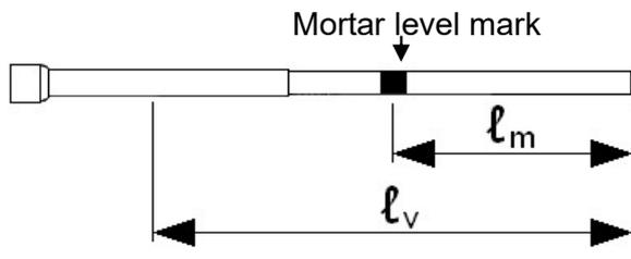
Mark the required mortar level  $l_m$  and embedment depth  $l_v$  with tape or marker on the injection extension.
