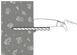
Any excess resin should be expelled from the hole evenly around the steel element showing that the hole is full. This excess resin should be removed from around the mouth of the hole before it sets.
