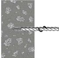
Insert the rebar, free from oil or other release agents, to the bottom of the hole using a back and forth twisting motion ensuring all the threads are thoroughly coated. Adjust to the correct position within the stated working time.
