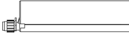
**Two part foil in a single piston component cartridge (FCC)**
