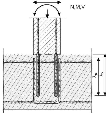
**Figure A3:** End anchoring of slabs or beams, designed as simply supported
