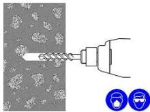
Drill hole to the required embedment depth using a hammer-drill with carbide drill bit set in rotation hammer mode, or a compressed air drill.
