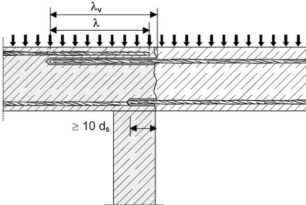
**Figure A2:** Overlap joint at a foundation of a column or wall where the rebars are stressed in tension
