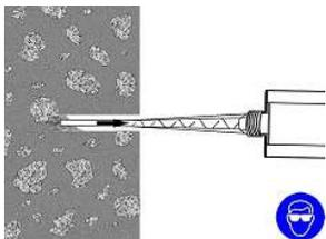
Insert the mixer nozzle (resin stopper / extension tube if applicable) to the bottom of the hole. Begin to extrude the resin and slowly withdraw the mixer nozzle from the hole ensuring that there are no air voids as the mixer nozzle is withdrawn. Fill the hole to approximately  $\frac{1}{2}$  to  $\frac{3}{4}$  full and remove the mixer nozzle completely.
