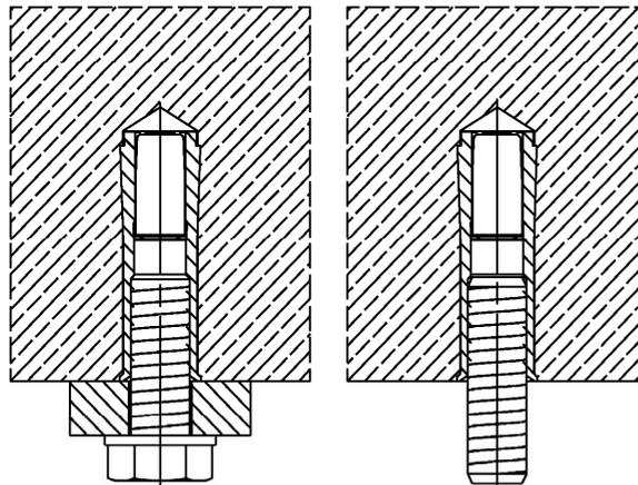
**Intended use in precast pre-stressed hollow concrete slabs ( $w/e \leq 4,2$ ) with a flange thickness  $d_b \geq 35$  mm (or 30 mm → see Annex C2) and only for  $h_{ef} = 25$  mm**
