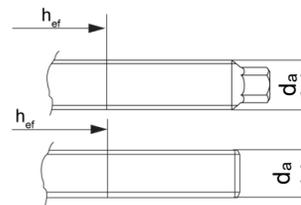
Alternative point geometry threaded rod
