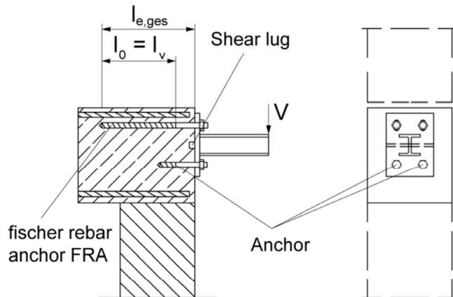
The required transverse reinforcement acc. to EN 1992-1-1:2004+AC:2010 is not shown in the figures. **The fischer rebar anchor FRA may be only used for axial tensile force.** The tensile force must transferred by lap to the existing reinforcement of the building. The transfer of the shear force has to be ensured by suitable measure, e.g. by means of shear force or anchors with European Technical Assessment (ETA)
