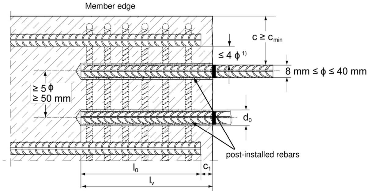
1) If the clear distance between lapped bars exceeds  $4\phi$  then the lap length shall be increased by the difference between the clear bar distance and  $4\phi$
