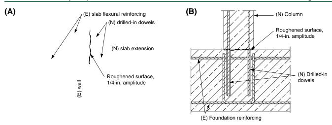
FIGURE 3— (A) OVERLAP JOINT WITH EXISTING REINFORCEMENT FOR REBAR CONNECTIONS (B) OVERLAP JOINT WITH EXISTING REINFORCEMENT AT A FOUNDATION OF A COLUMN OR WALL
