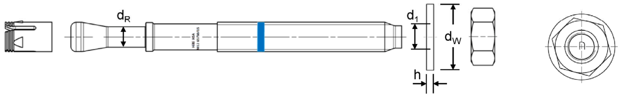
Figure A2: Hilti metal expansion anchor HSA-BW
