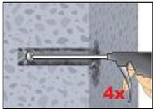
The hand-pump can be used for anchor sizes up to bore hole diameter 20 mm.
