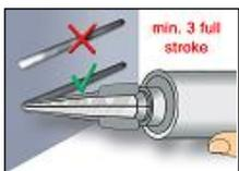
5. Prior to dispensing into the drill hole, squeeze out separately a minimum of three full strokes and discard non-uniformly mixed adhesive components until the mortar shows a consistent grey or blue (PYSF Change) colour. For foil tube cartridges it must be discarded a minimum of six full strokes.
