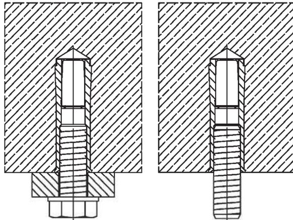
**Intended use in precast prestressed hollow concrete slabs ( $w/e \leq 4,2$ ) with a flange thickness  $\geq 30$  mm and only for  $h_{ef} = 25$  mm**
